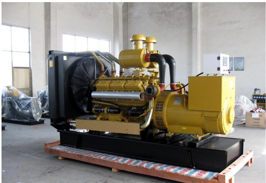
genset in the workshop
