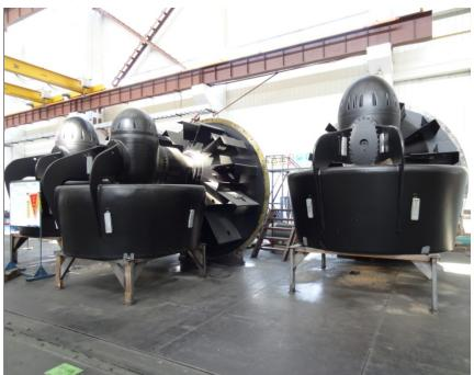
**Well installation** is especially for tugs, ferries, well station, floating dock and survey ships.
