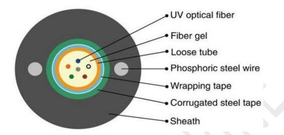
Unitube light armored fiber optic cable GYXTW construction
