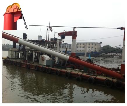
The dredge anchor boom'length depends on the stability and the dimensions of the pontoon. It can determines how far the anchor can be placed outside the Cutter Suction Dredger.
